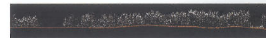
▲ Recording multiple laser-pulse returns enables separation of forest canopy from bare ground using proper filtering techniques accompanied by manual editing.
